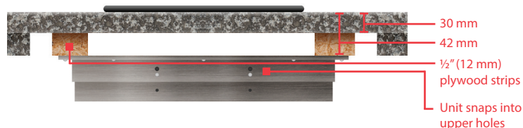
Figure 3: Incogneeto™ Unit Mounted to 1¼" (30 mm) Countertop with Two Plywood Strips
